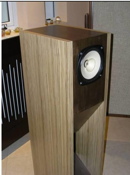
95 db/W/m - 8 Ω - FOLDED HORN
