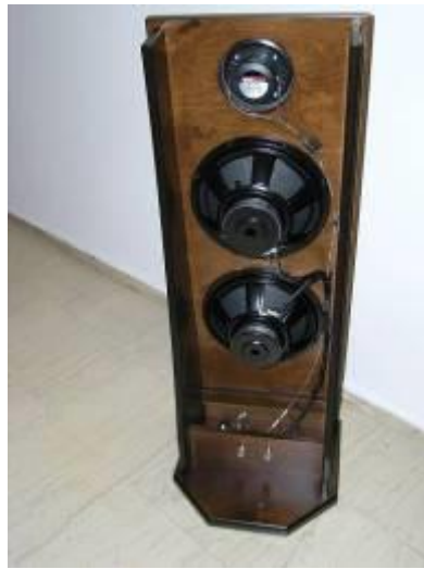
90 db/W/m - 6 Ω - 150 Watt - Programm 2 Woofers 12 `` - Tweeter 30 mm Wave Guide .
